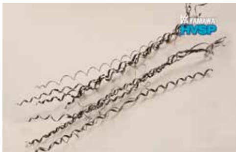
Ejected chips by large size taps
