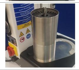
Push the tool holder into the cooling position. Cooling is started automatically via a switch.
