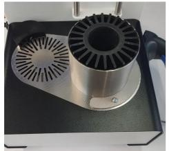
Place the appropriate setting pot in the shrink position under the coil.
