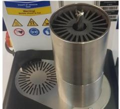
For safe cooling after tool change, a matching cooling adapter is fitted over the tool holder.
