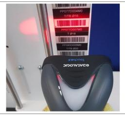
Use the handheld scanner to scan the appropriate barcode for the tool holder (see 4.6.3) to set the operating parameters for the next shrink operation.
