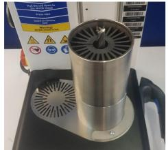
For safe cooling after tool change, a matching T3-K cooling adapter is fitted over the tool holder.
