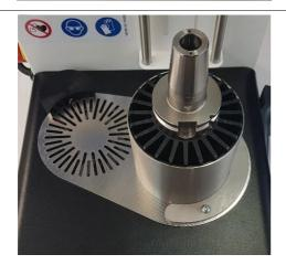
Insert the tool holder into the setting pot.
