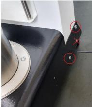
Larger deviations must be adjusted via the lateral screws on the generator housing.
