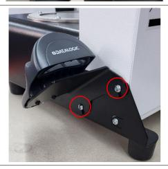
Loosen the two marked screws until you can insert them into the slots in the scanner holder.
