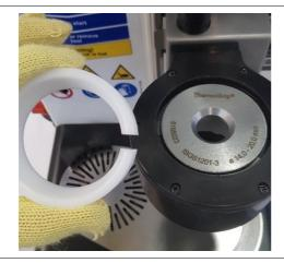
To remove the disk, compress the white plastic clamping ring manually.
