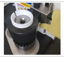
Position the coil on top with the tool holder.
